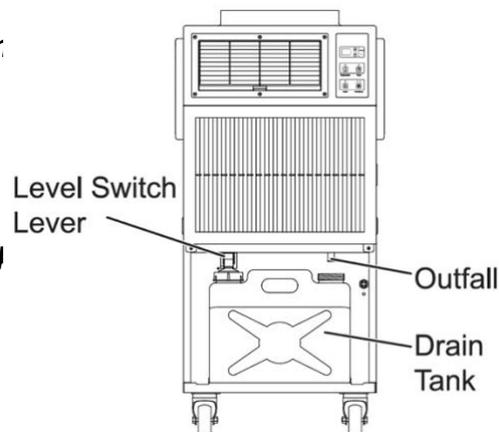
***Note: The condensed water can be directly discharged through a gravity drain. Remove the drain tank, connect the drain outlet directly to the machine through the bottom side discharge hose or out through the right-side discharge hose outlet.***
